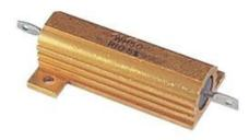
We are talking here about chassis-mount resistors with built-in heatsinks. These are by far the most efficient means of dissipating power, provided that the heatsink (or fan) is adequate. Heatsink compound should be used, and fasteners should include lockwashers or kepnuts.
