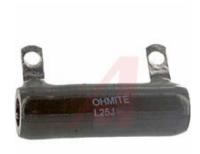
25W power resistors have flat mounting tabs that are designed to transfer heat more efficiently than a wire lead. These tabs can transfer prodigious heat, and precautions must be taken when mounting on terminal strips.
